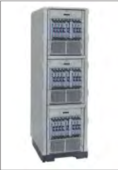
Figure 5. Three fully configured HP Blade Server bh7800 Chassis in a rack
