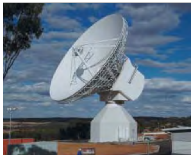
Figure 3. Antenna system for TT&C
