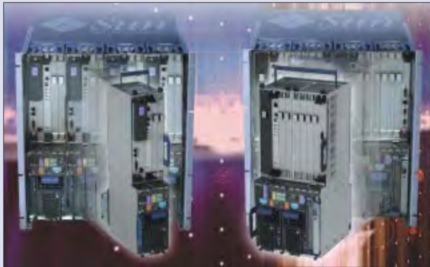
Figure 2. Netra CP2060 CompactPCI with PMC I/O expansion
